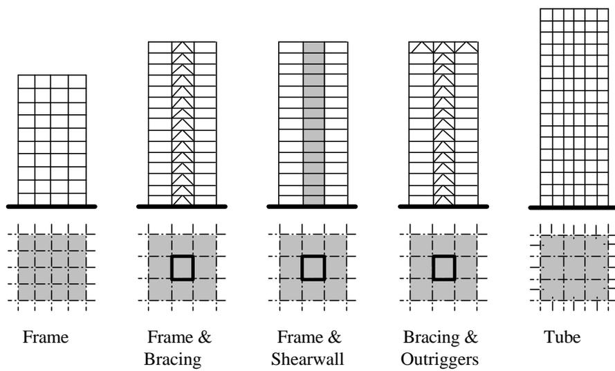
**Figure 1: Structural system types**
