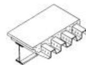
h) Composite steel beam & deck & concrete slab
