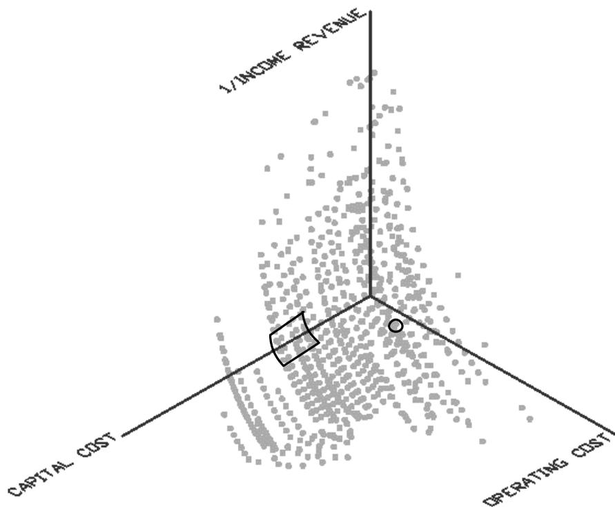
**Figure 4: Optimal cost-revenue trade-off surface**
